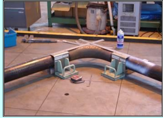
Figure 9. Conventional dimensional inspection of bended pipe. Measuring length between intersections using measurement tools.
