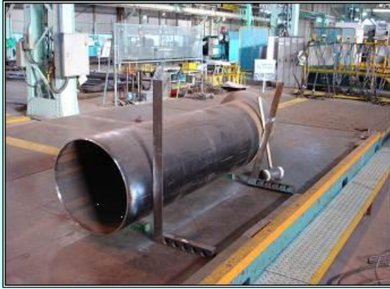
Figure 8. Conventional dimensional inspection of bended pipe. Setting on the surface plate.
