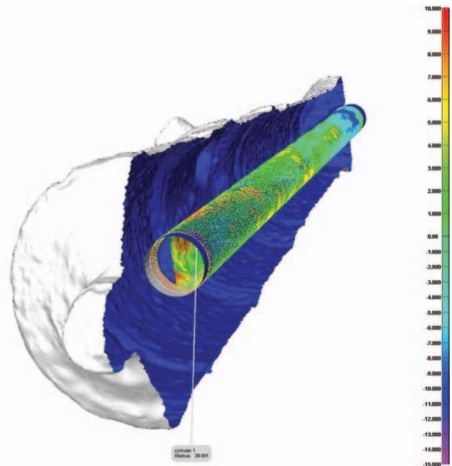
Figure 16. Bore taper viewed from chamber
