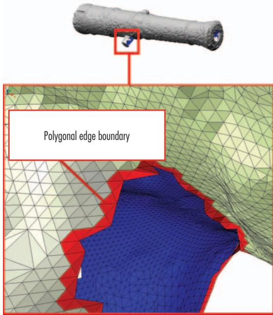
Figure 14. Polygon edges are used to detect and fill holes.
