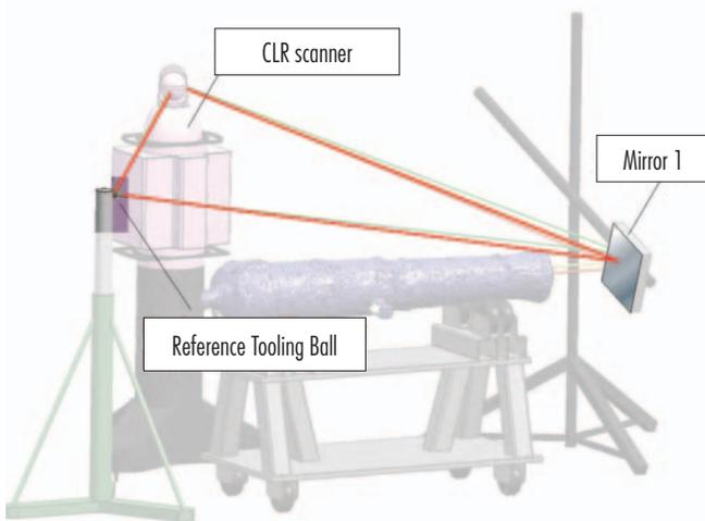
Figure 6. Position of key measurement components
