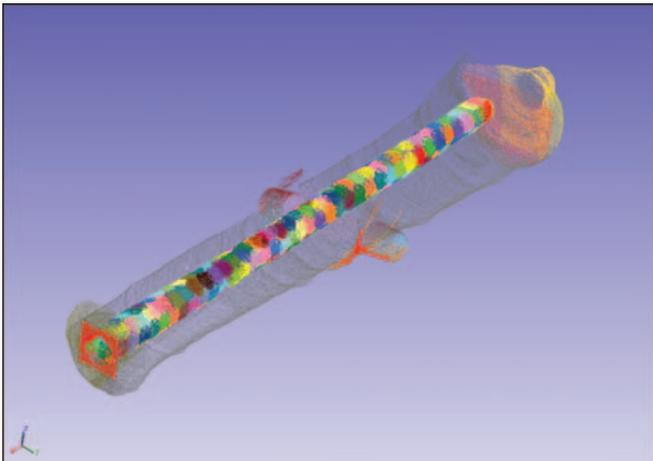
Figure 12. Full bore coverage required a patchwork of point clouds
