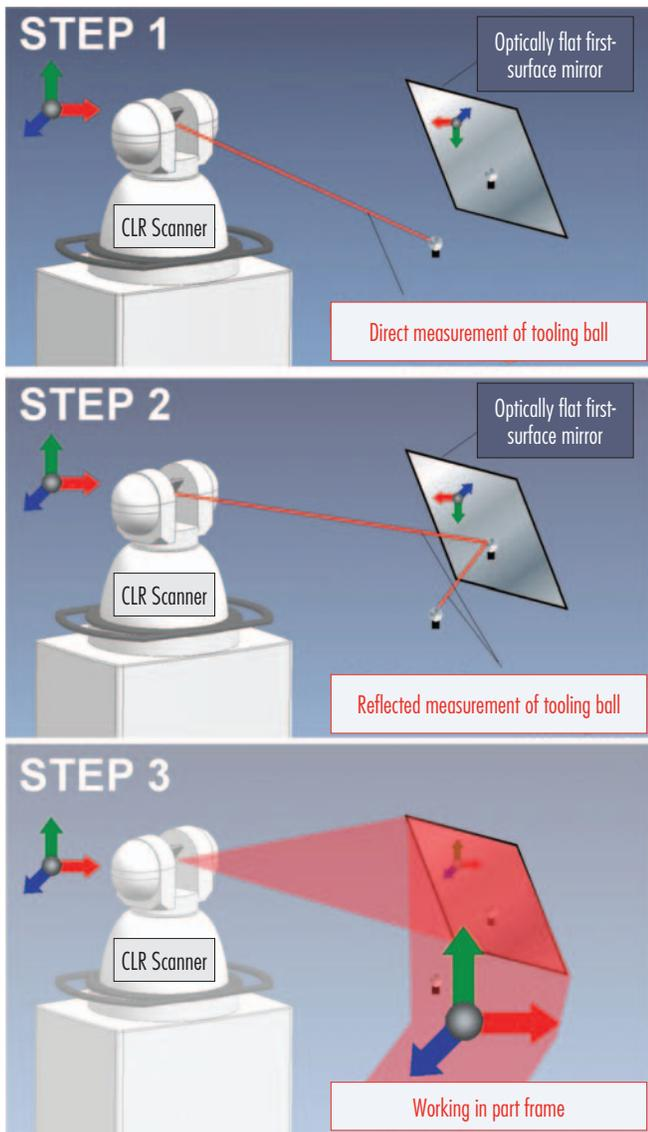
Figure 5. Transforming reflected images into working reference frame
