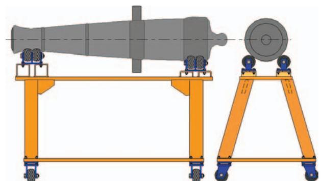
Figure 7. Cannon roller support assembly
