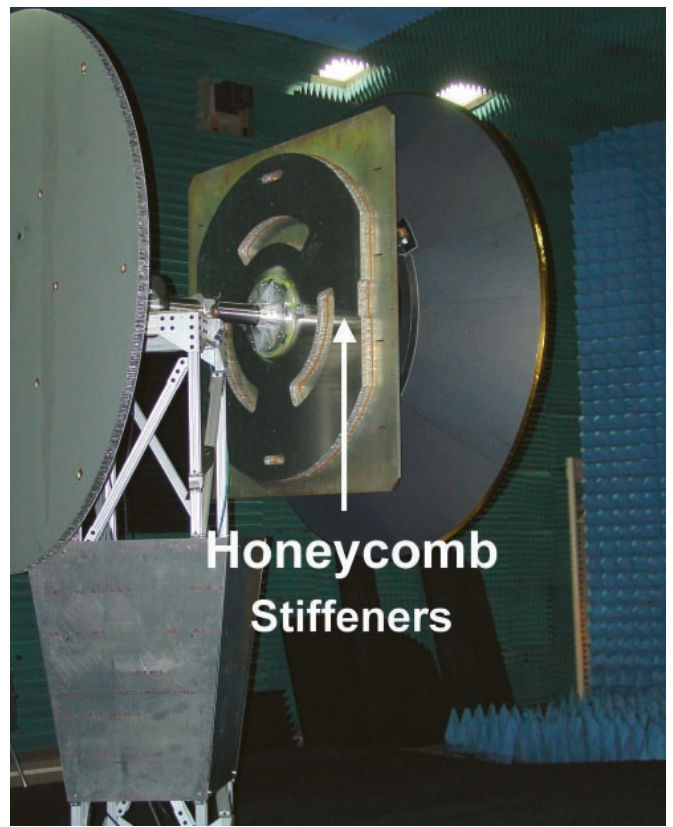
Figure 20. RF test stand with stiffened backing plate.
