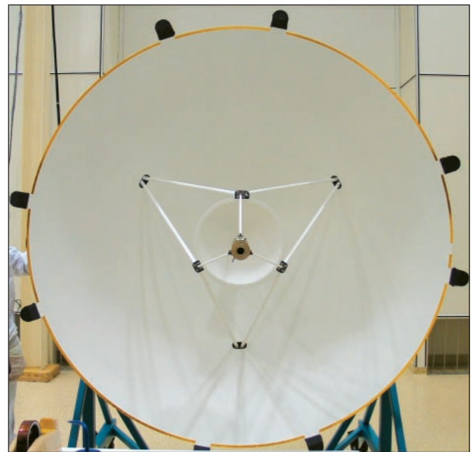
Figure 8. Actual HGA, as delivered, with tooling ball "ears" around circumference.
