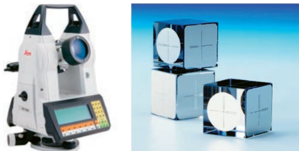
Figure 9. Leica T5100A autocollimating theodolite 2 (left) and reference optical cubes 3 (right).
